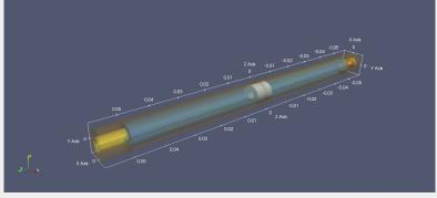
The material under test (MUT) was placed in the center.
